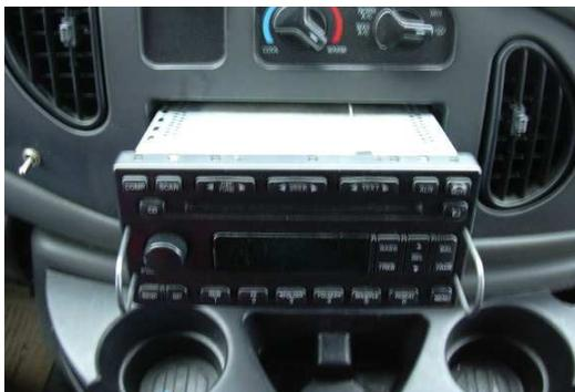
**Step 6** Disconnect the factory stereo
