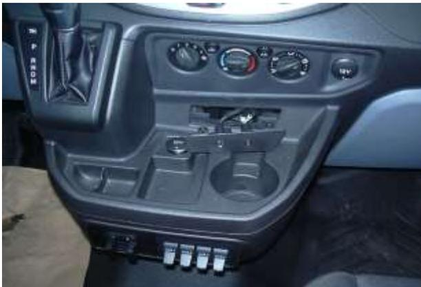
**Step 2** Unclip the 3.5 socket assembly from the plate, you might need to insert a small blade to release the clips. **Use caution!**
