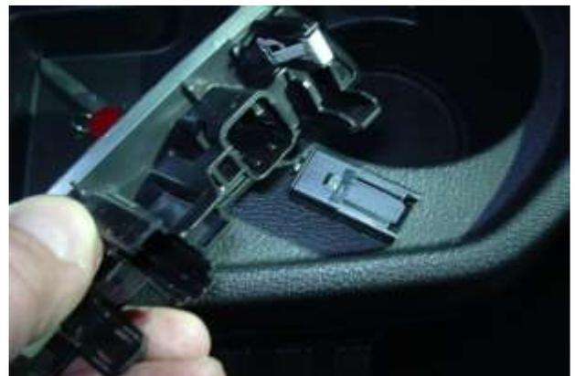
**Step 3** Unclip and lift off the drink tray vertically to expose the power port power connection plug.
