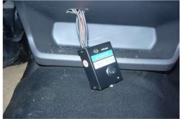
**Step 5** Using crimp connectors, connect the red wire on the PA to the gray and the black PA wire to the black with blue stripe. Fish the PA output wire and connect to the AUX input socket. Tape the connection to make sure it never comes undone.
