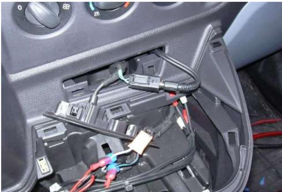
**Step 6** Now it's time to test the operation of the PA system. Turn on the key, put the stereo into the "Sync Input" mode, set the volume to about 16 -17 and talk into the mic. Once tested, reconnect the power port plug and re-install the drink tray, then re-install the plate for the USB. Clean the back of the PA box and the underside of the console with rubbing alcohol to remove any film, let dry and install the Velcro and push firmly in place.
